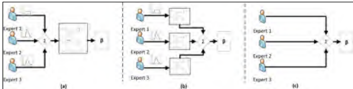
Figure 3.1 Different configurations of expert opinions fusion: (a) Fusion before propagation into the system model-(b) Fusion after propagation into the system model- (c) Experts directly provide model output
