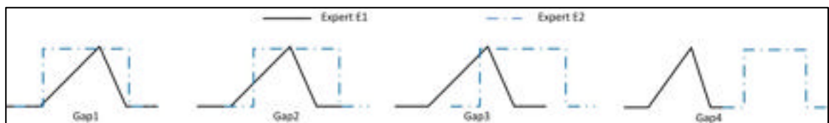
Figure 3.9 Illustration of the 4 considered gaps between 2 experts. In this example the opinion of expert E_1 follows a triangular distribution and the opinion of expert E_2 follows a uniform distribution
