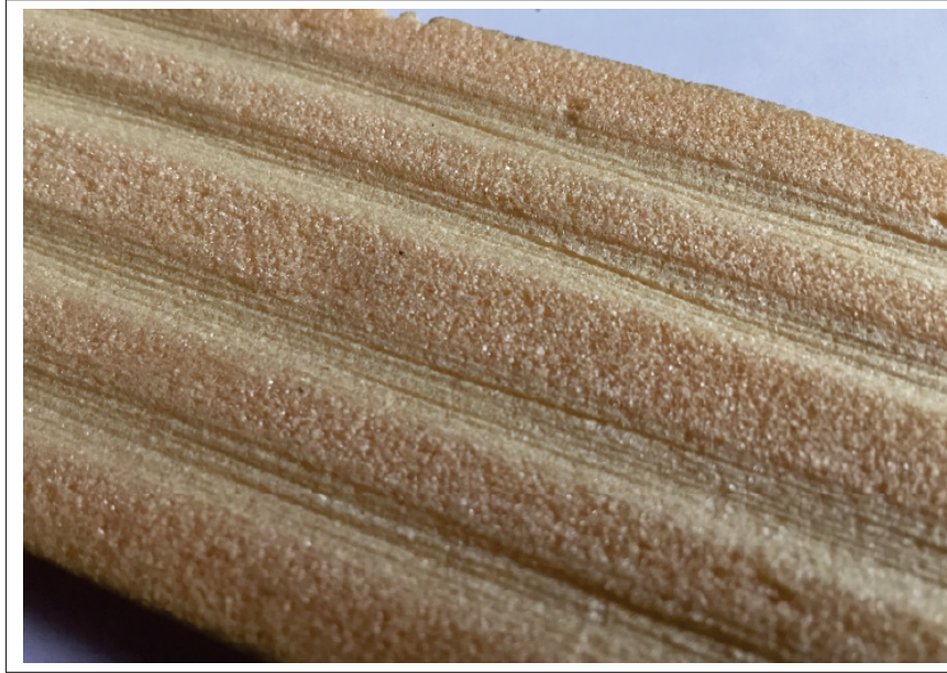
Figure 3.37 Foam Core damage from SMA wires
