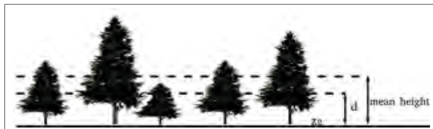
Figure 2.1 Representation of the elevation in the displacement height model. Figure adapted from Stull (1988)
