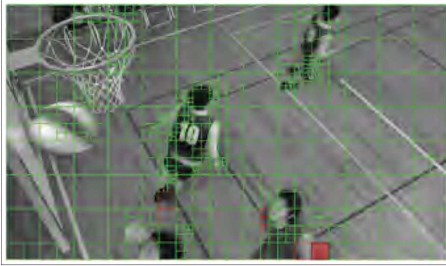
Figure 1.5 Frame partitioning with the quadtree coding blocks
