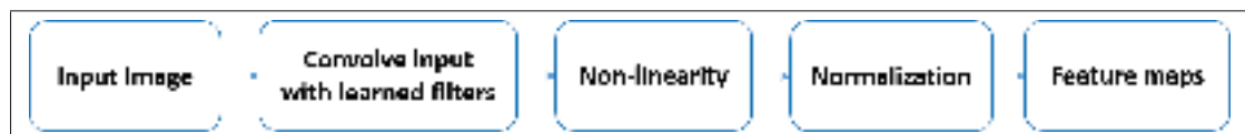
Figure 4.2 Feature Extraction Using Convolutional Neural Networks (CNNs): Convolutional operation is performed by moving the filters with fixed stride through the input image and computing the convolution between each filter matrix and input image matrix. Non-linearity is introduced after each convolutional operation by applying a Rectified Linear Unit (ReLU) since convolution is a linear operator. Features are extracted from the fully connected layer right before the classification layer.
