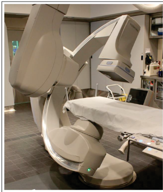
Figure 1.7 Single axis rotational X-ray angiography in CHU Sainte-Justine.
