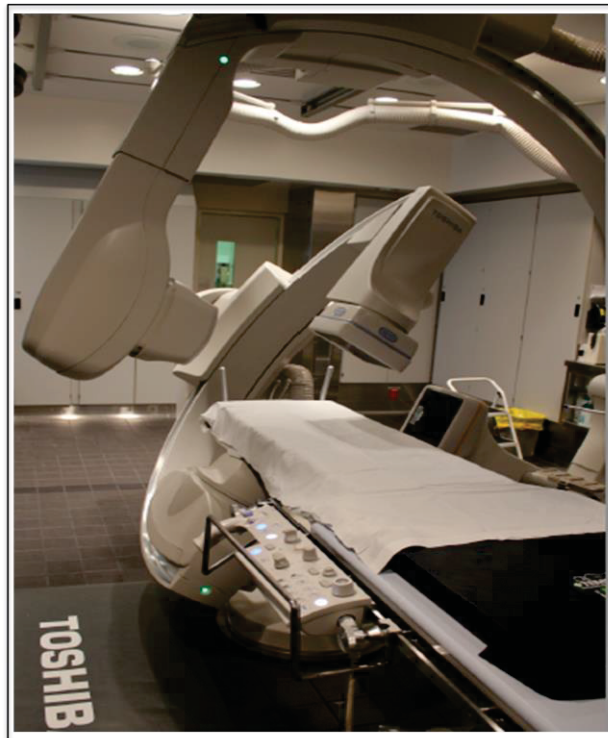
Figure 1.8 Dual axis rotational X-ray angiography in CHU Sainte-Justine.
