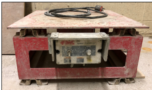
Figure 5.6 Plaque vibrante Syntron VP-51
