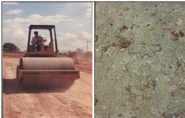
Figure 1.46 Microfissuration de la base traitée (Scullion, 2002)
