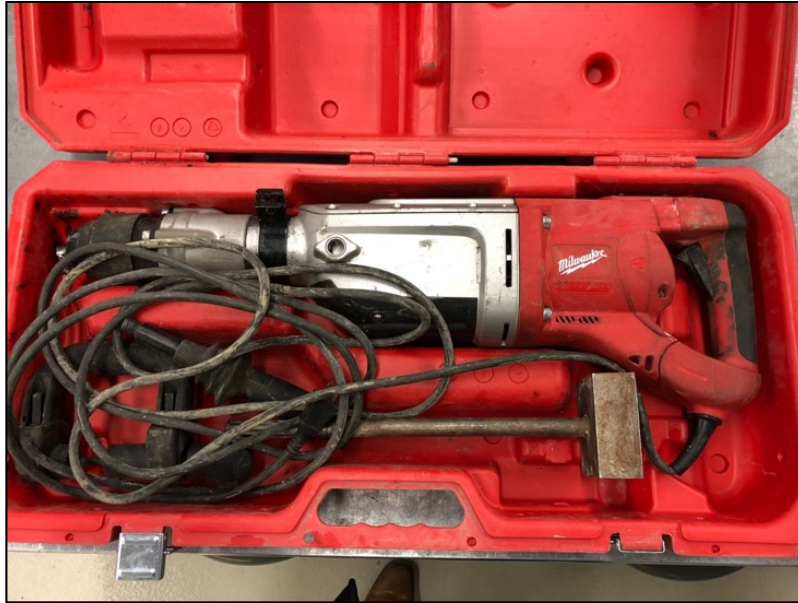
Figure 5.11 Marteau mécanique Milwaukee SDS-MAX 50 mm (# 5229-21)
