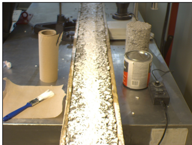
Figure 5.23 Application de la pellicule de fissuration
