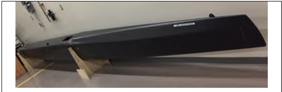
Figure 5.12 Coque tribord collée (avant finition)
