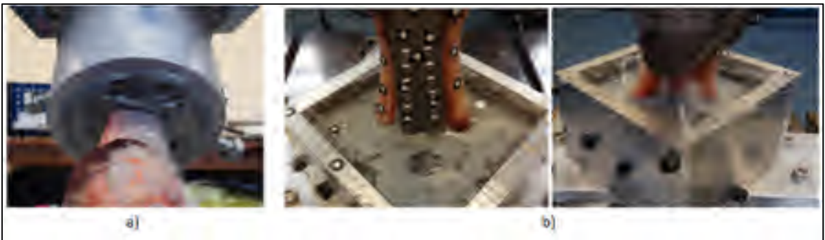
Figure 2.13 : Bone extremities embedded in polyurethane resin: a) humerus, b) metacarpals
