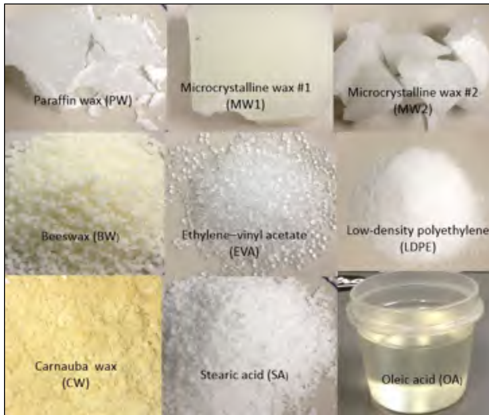
Figure 3.2 Appearance of the binders used in our study at room temperature.
