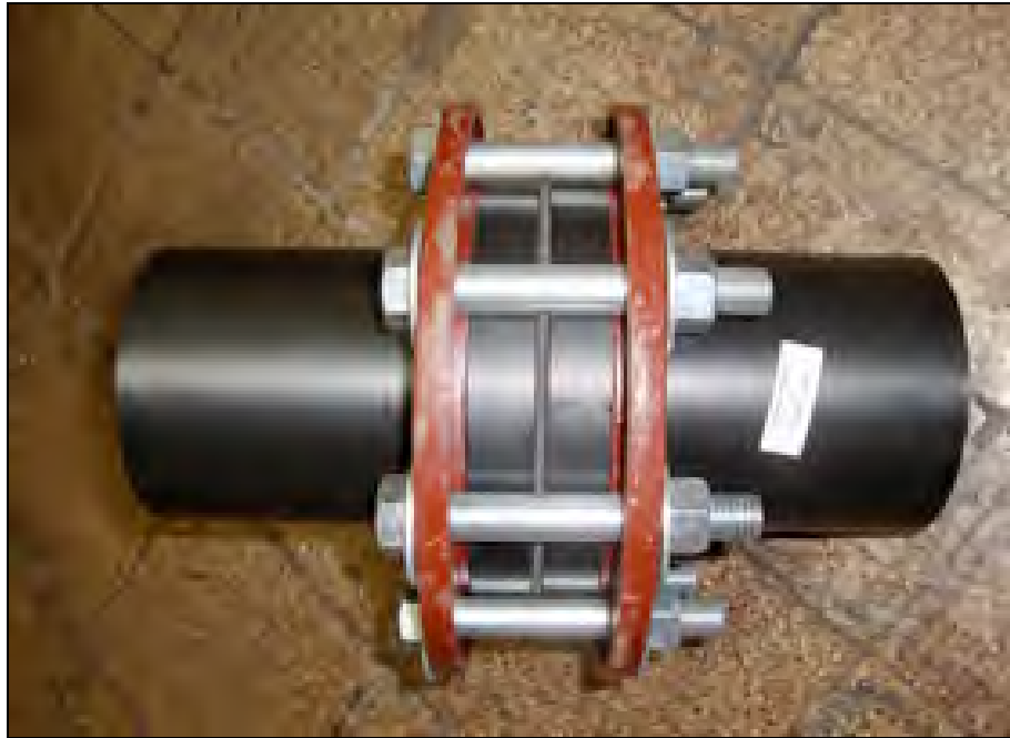
Figure 0. 2 HDPE Bolted Flange joint
