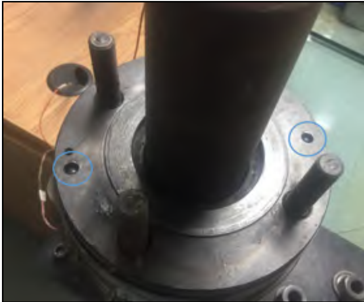
Figure 2. 12 HOBT displacement measurement system
