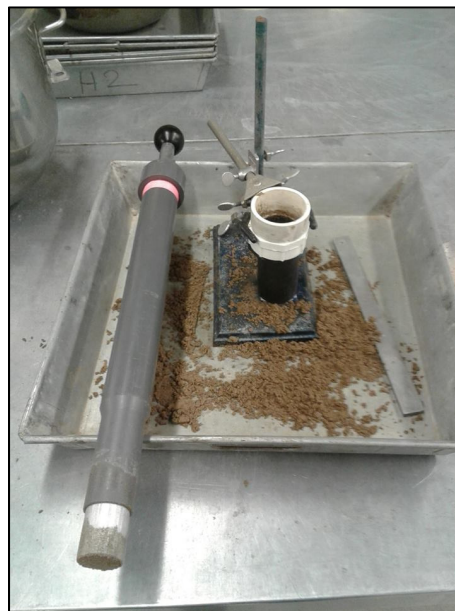
Figure 2-5 Marteau de compactage
