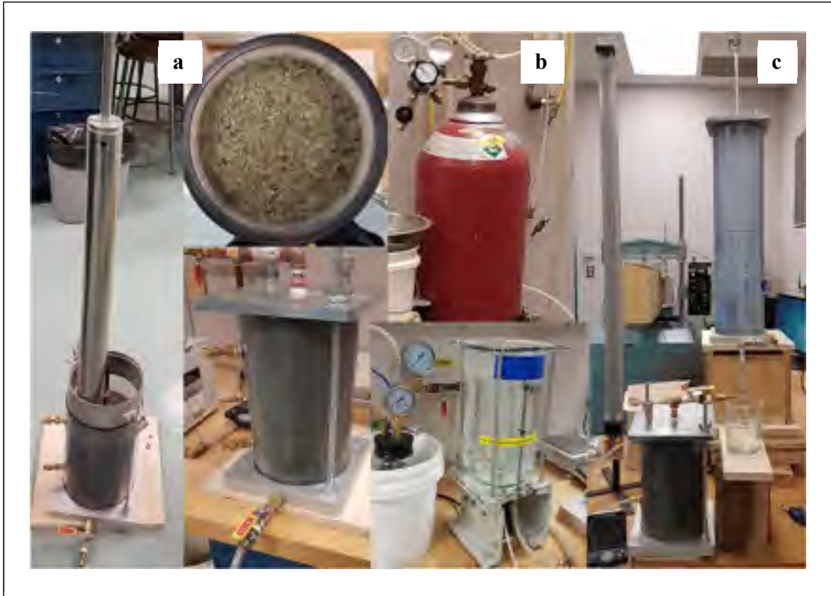
Figure 2-2 (a) Compaction step and prepared samples for saturation step (b) saturation of specimens from bottom upward with de-aired water after expelling the adhered oxygen by CO 2 (c) hydraulic conductivity test based on constant-head method
