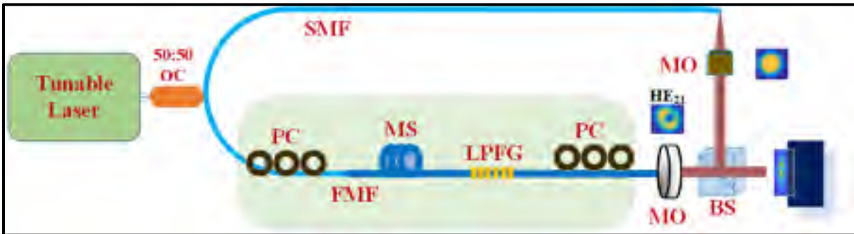
Figure 4.5 Experimental setup for the generation and detection of OAM beams
