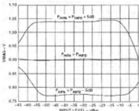
TPC 12. VMAG Output vs. Input Level for  $P_{\text{DNR}} = P_{\text{DFS}}$ ,  $P_{\text{DNR}} = P_{\text{DFS}} + 5$  dB,  $P_{\text{DNR}} = P_{\text{DFS}} - 5$  dB. Frequency 1900 MHz
