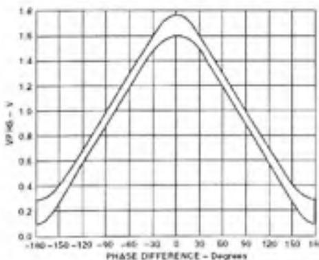
TPC 33. Distribution of VPHS vs. Input Phase Difference, Three Sigma to Either Side of Mean, Frequency 900 MHz, Temperature between  $-40^{\circ}\text{C}$  and  $+85^{\circ}\text{C}$ , Input Levels  $-30$  dBm
