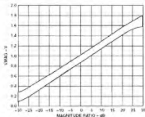
TPC 10. Distribution of VMAG vs. Input Level Ratio (Gain). Three Sigmas to Either Side of Mean. Frequency 1900 MHz, Temperatures Between  $-40^{\circ}\text{C}$  and  $+85^{\circ}\text{C}$ , Reference Level =  $-30$  dBm
