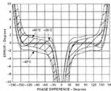
TPC 32. Distribution of VPHS Error vs. Input Phase Difference, Three Sigma to Either Side of Mean, Frequency 2200 MHz,  $-40^{\circ}\text{C}$ ,  $+25^{\circ}\text{C}$ , and  $+85^{\circ}\text{C}$ , Input Levels  $-30$  dBm
