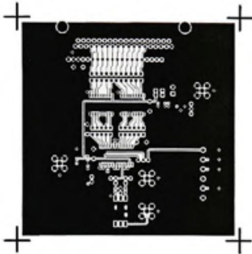
Figure 12. Printed Circuit Board Top Side Copper
