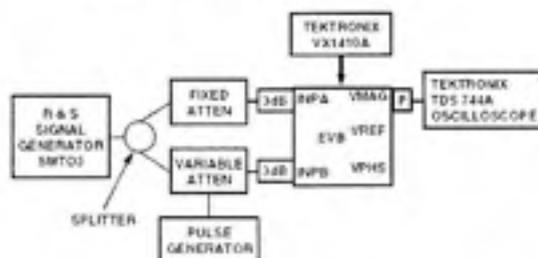
Figure 17. VMAG Dynamic Performance Measurement Setup
