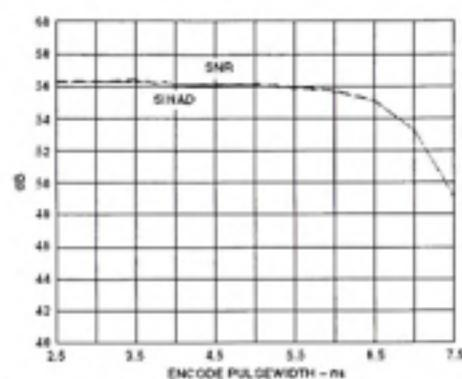
TPC 9. SNR vs. Clock Pulsewidth ( $t_{cp}$ );  $f_{IN} = 10.3$  MHz
