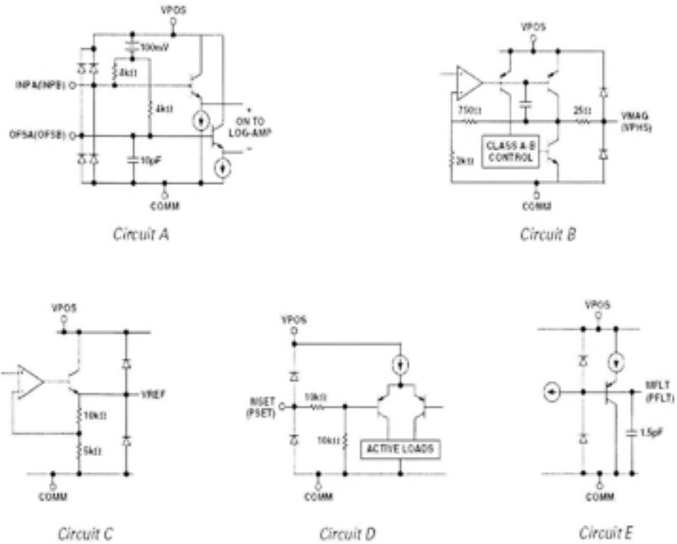
Figure 1. Equivalent Circuits
