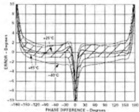
TPC 30. Distribution of VPHS Error vs. Input Phase Difference, Three Sigma to Either Side of Mean, Frequency 900 MHz,  $-40^{\circ}\text{C}$ ,  $+25^{\circ}\text{C}$ , and  $+85^{\circ}\text{C}$ , Input Levels  $-30$  dBm
