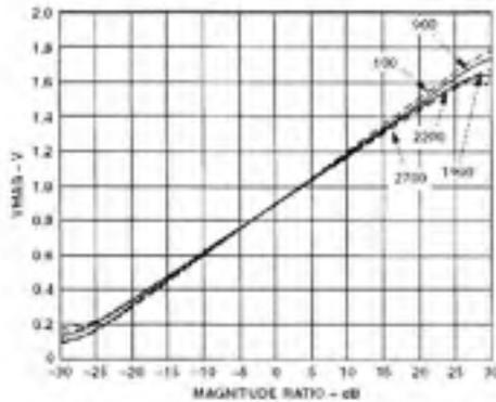
TPC 1. Magnitude Output (VMAG) vs. Input Level Ratio (Gain).  $V_{REF} = V_{IN}$ . Frequencies 100 MHz, 900 MHz, 1900 MHz, 2200 MHz, 2700 MHz, 25°C,  $P_{IN} = -30\text{ dBm}$ , (Re: 50  $\Omega$ )
