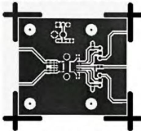
Figure 15a. Component Side Metal of Evaluation Board
