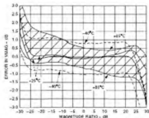
TPC 8. Distribution of Error vs. Input Level Ratio (Gain). Three Sigmas to Either Side of Mean. Frequency 1900 MHz,  $-40^{\circ}\text{C}$ ,  $+25^{\circ}\text{C}$ , and  $+85^{\circ}\text{C}$ , Reference Level =  $-30$  dBm
