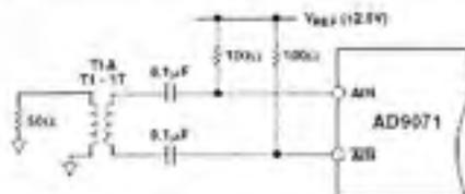
Figure 7. Differential Analog Input Configuration
