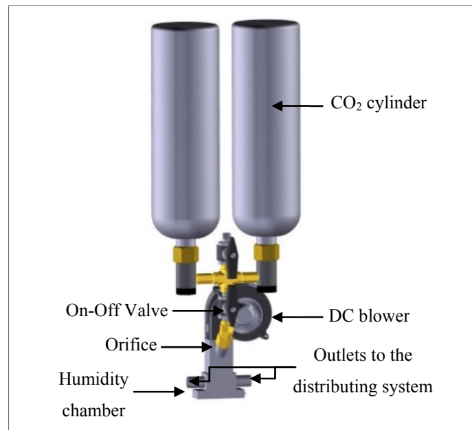
Figure 4.1 \text{CO}_2 distribution and air-treating systems
