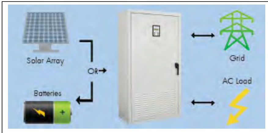
Figure 6-15 Schematic of Battery Inverter to AC Load or Grid [6] Taken from Princeton Power System GTIB-480-125 (2017)
