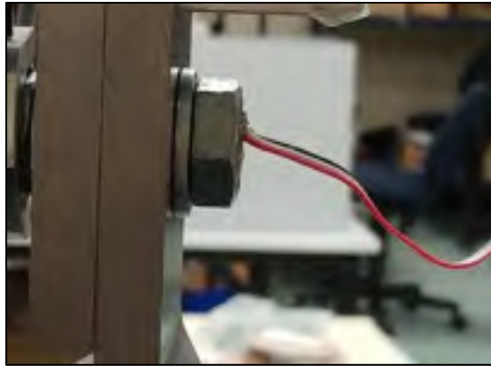
Figure 2-15 Strain gage installed in the bolt
