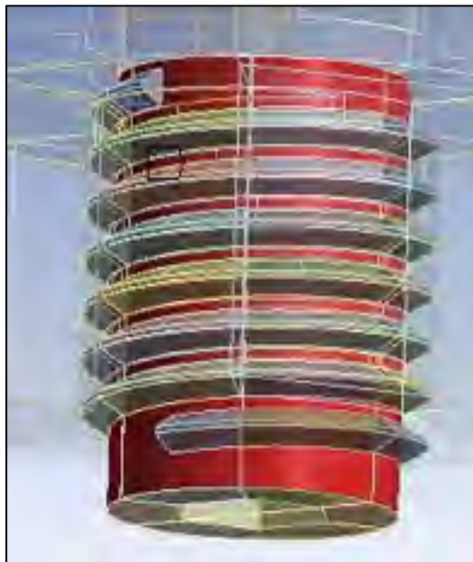
Figure 3-17 Bonding surfaces of the bolt threads and stem
