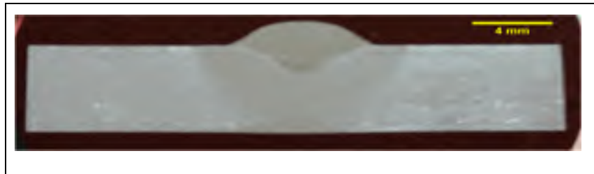
Figure 2.6 Polished and etched sample for microstructure characterisation extracted from horizontally welded plate
