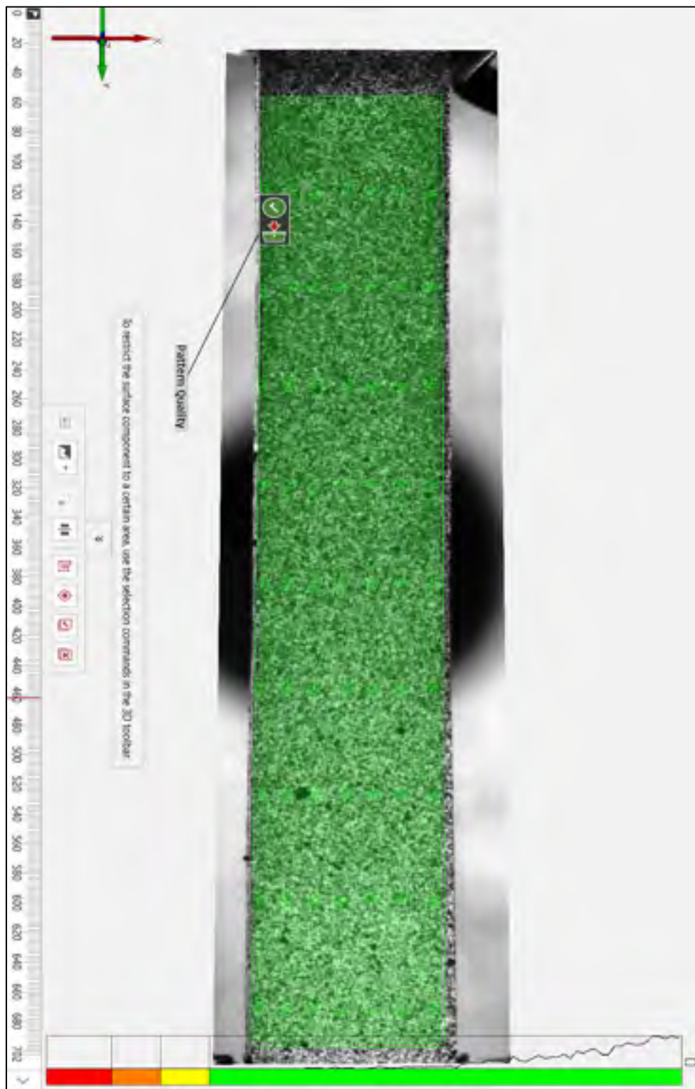
Figure-A IV-5 Speckle pattern quality in DIC
