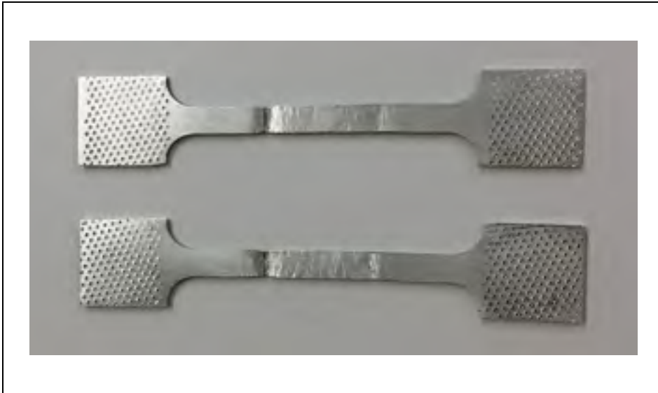
Figure-A IV-3 Fracture of MFT specimens DIC test
