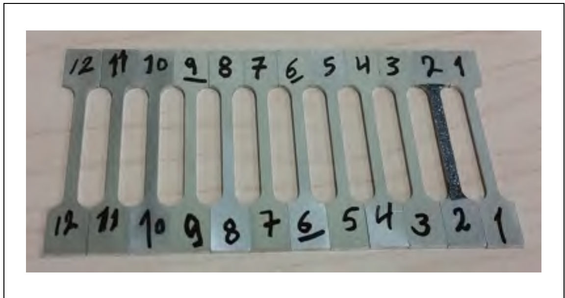
Figure-A IV-2 MFT extracted specimens
