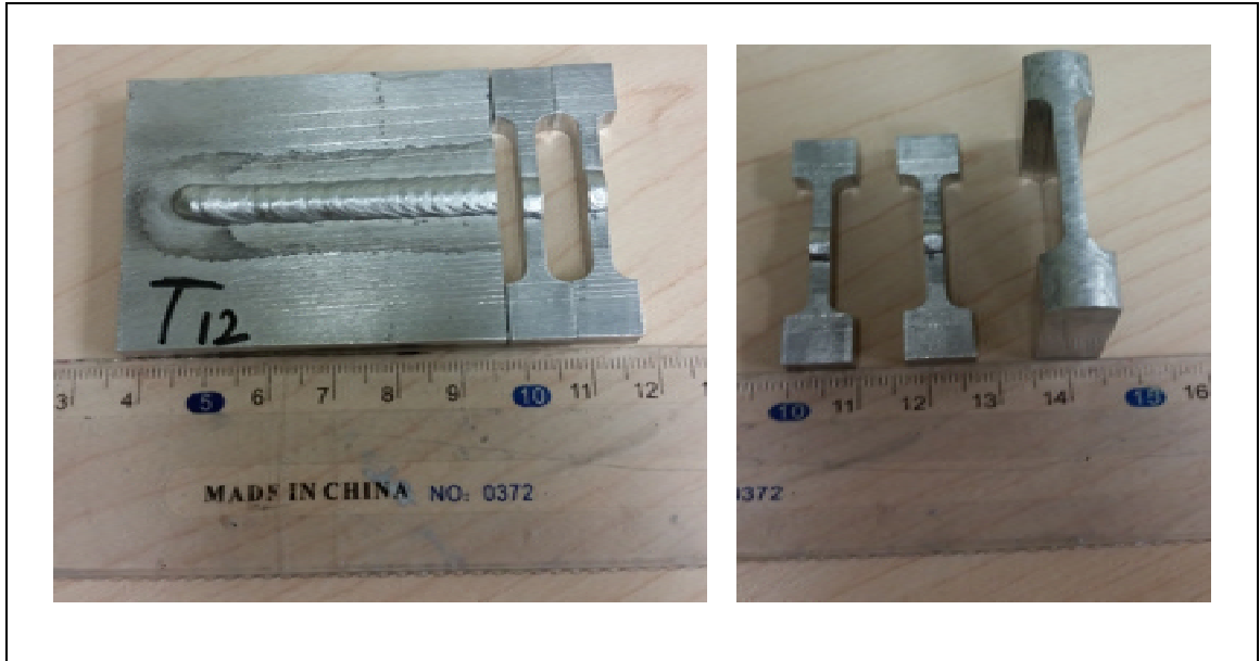
Figure-A IV-1 MFT specimens extracted from welded samples
