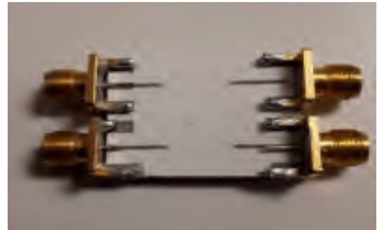
Fig. 4. Photo of prototype of Microstripline-to-buried line-to- Microstripline.
