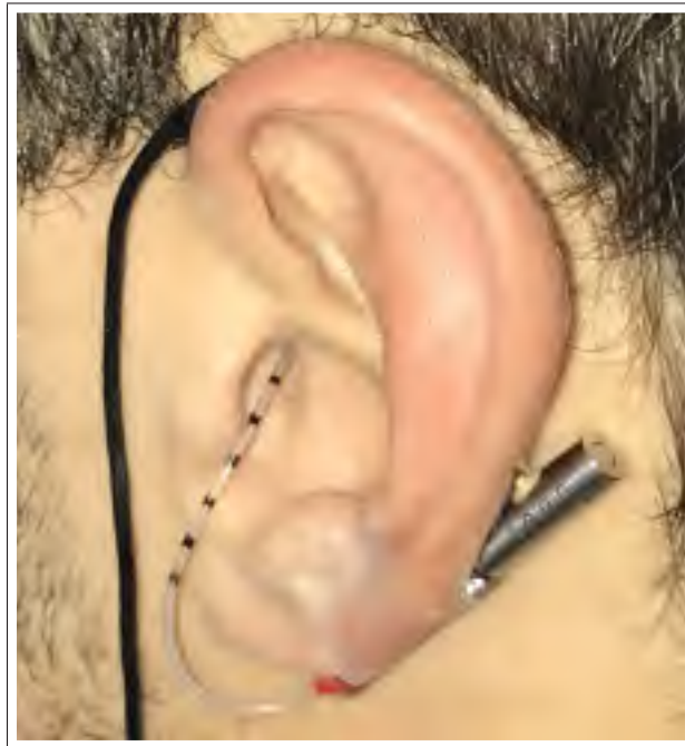
Figure 3.7 Apparatus used for in-ear measurements. A small microphone was taped behind the participant's ear and connected to the probe tube inserted within the ear canal. Black marks made at every 4 mm on the probe tube allowed the experimenter to perform acoustic pressure measurements at approximately every 2 mm, from eardrum to ECE
