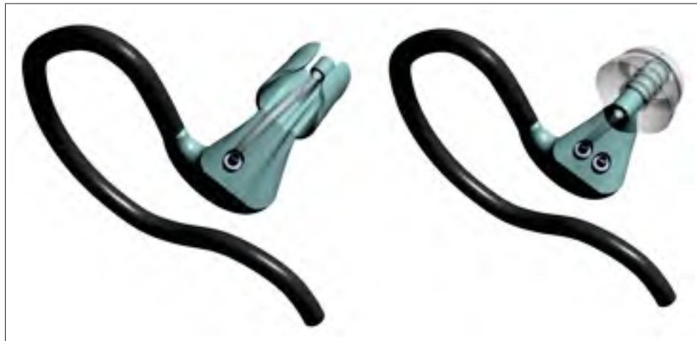
Figure 2.3 (Color online) Three-dimensional models showing the OTE (left) and the CTE (right). In-ear measurements are performed via thin probe tubes connected to miniature electret microphones. An outer-ear microphone (OEM) on the CTE makes it possible to measure earplug attenuation
