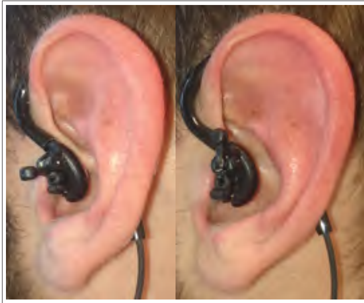
Figure 3.20 Dosimetric earplug, as worn with the vent in open (left) or sealed (right) conditions
