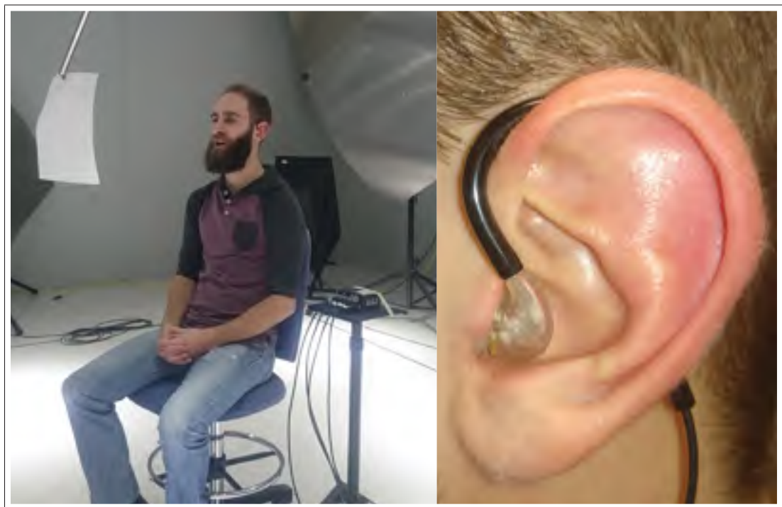
Figure 4.3 Left : Subject speaking while seated in the reverberant room, as part of the experimental procedure. Subject is wearing the earpiece shown in Fig. 4.1 and pronounces phrases written on the sheet in front of him. White noise is played simultaneously on the four loudspeakers. Right : picture showing the earpiece as worn in the participant's ear
