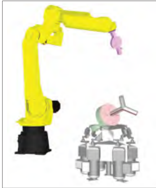
Figure 2.21 The final placement of the rotary table on the hexapod. It is not conventional to place the rotary table with an orientation to the surface of the EE. A spacer is needed in this situation in order to place and fix the rotary table on the hexapod.
