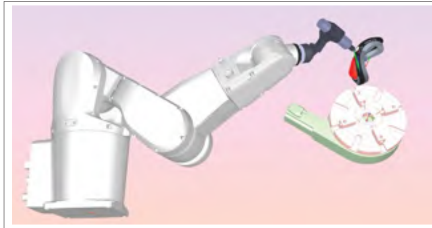
Figure 3.10 The final configuration of the coordinated robotic system to glue the ski goggles, using a rotary table as the RP.
