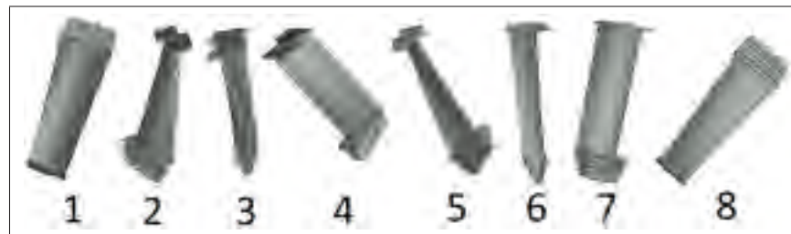
Figure 4.6 Eight images needed to be taken from different angles of the turbine blade for the sake of inspection.
