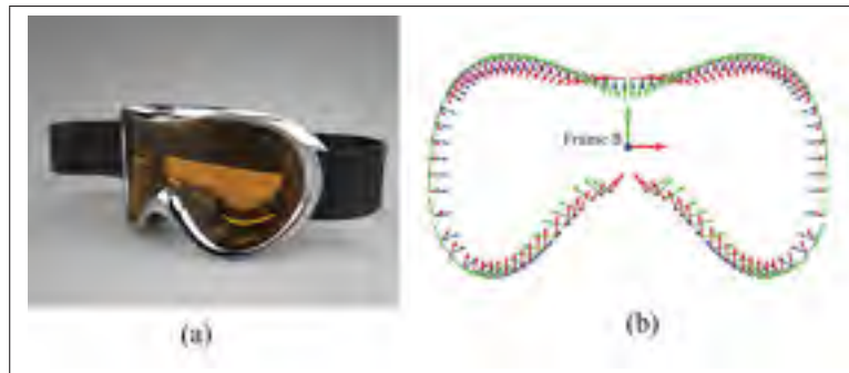
Figure 3.1 (a) Ski goggles; (b) ski goggles path used throughout this chapter as an example. Each point of the path is a frame (origin and orientation). Red, Green and Blue (RGB) are x , y and z axes, respectively.
