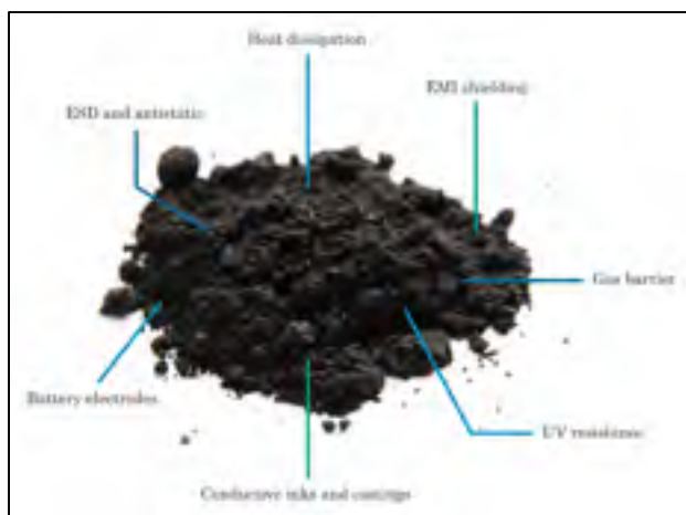
Figure 2.3 The application of graphene black 3X in the industry (Technical data sheet from NanoXplore)
