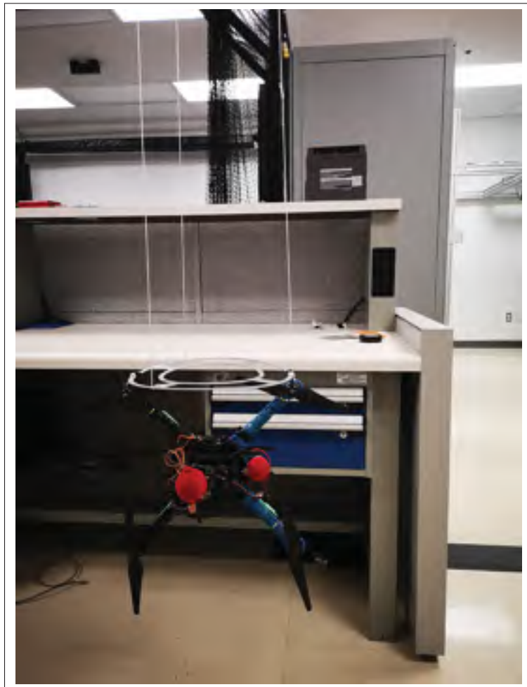
Figure 2.6 Measurement of Mass Moment of Inertia along y-axis
