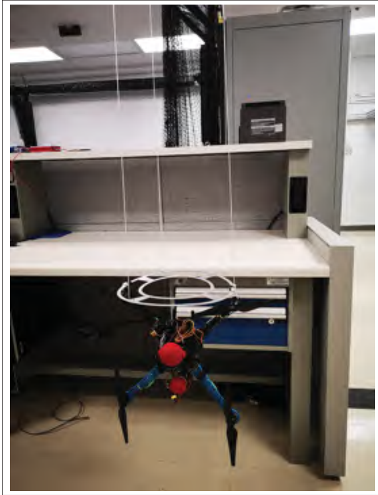
Figure 2.5 Measurement of Mass Moment of Inertia along x-axis
