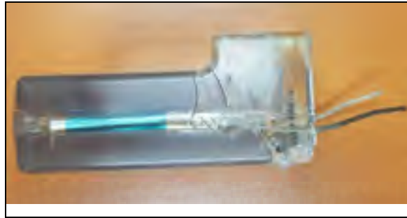
Figure 4.11 Fissurations sur VPI 23
