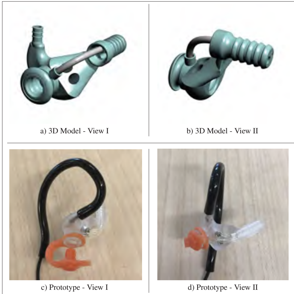
Figure 2.14 Details of a temporary CEP prototype using a silicone cap to close the vent
