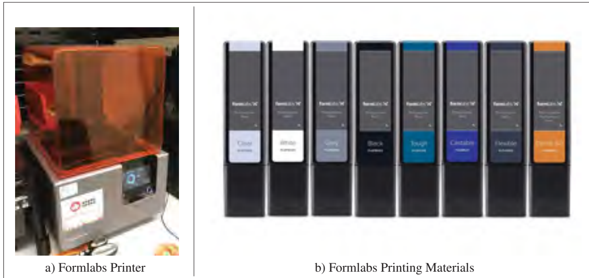
Figure 2.7 Formlabs printer and resin options Adapted from Formlabs (2019)
