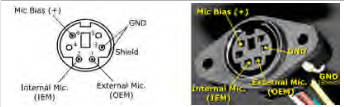
Figure-A III-4 Mini-DIN6-F pinout (front view)
