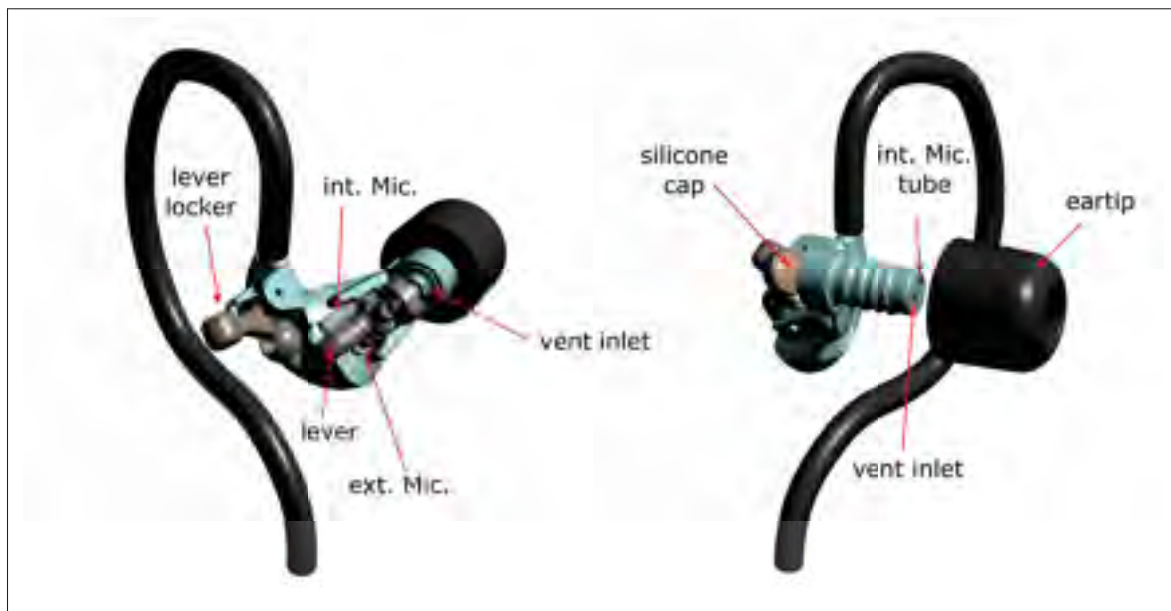
Figure 2.15 3D rendering model details of the closed-earpiece device
