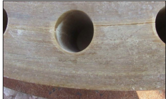
Figure 1-25 Crack in the flange face between the bolts and inside the bolt hole (Dynaflow 2011)
