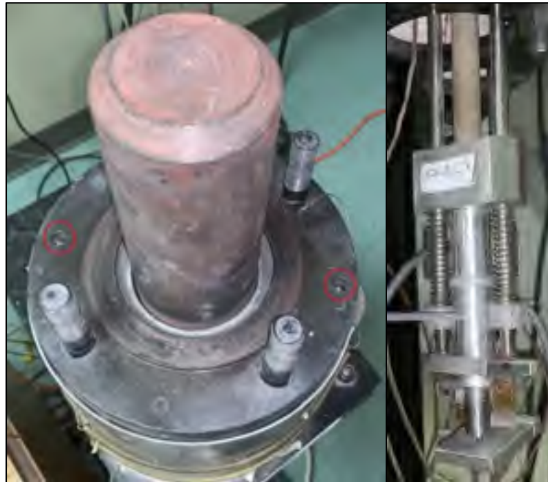
Figure 4-4 HOBT displacement measurement system
