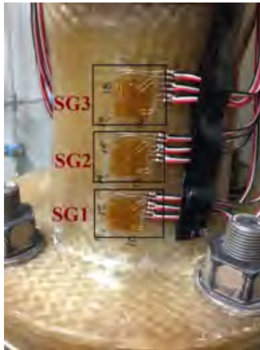
Figure 4-5 Strain gauges attached on FRP flange
