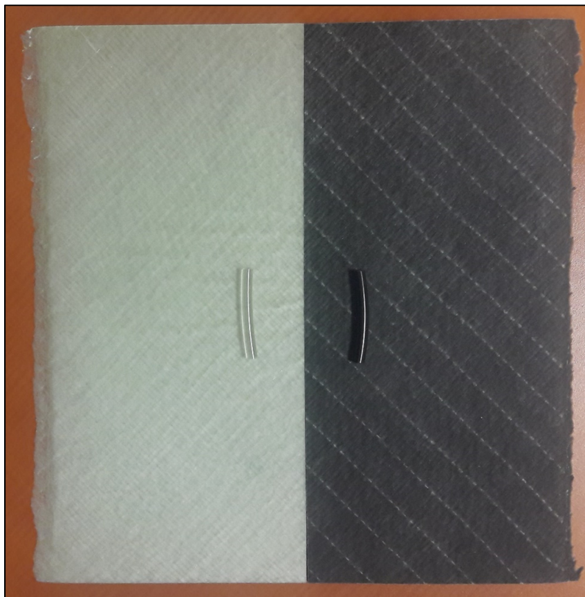
Figure 3.2 Plaques with net epoxy (left) and 1 wt% graphene addition to epoxy (right) and their respective epoxy
