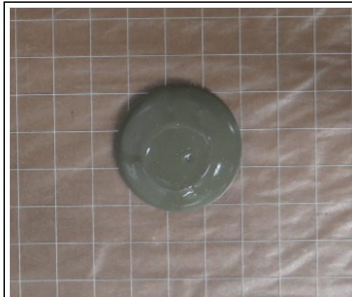
Figure 2.6 Presence of a "hat" after conducting the mini-slump test for mix 12
