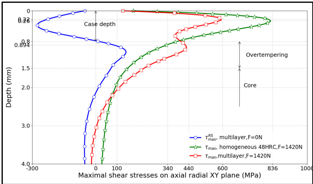
Figure 3-10 Maximal shear stress on axial radial XY plane, in multilayer without load (blue line), and under a 1420 N loading case (red line); compared with homogenous case under a maximal loading of 580 N (green line)
