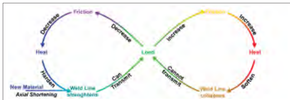
Figure 1.4 Linear Friction Welding (LFW) self-regulating cycle
