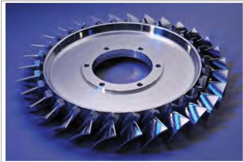
Figure 1.1 LFW blisks assembly made by The Welding Institute (TWI (2018))
