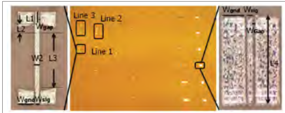
Figure 0.17 Aerosol Jet Printed CB-CPW-MS transmission line Cai et al. (2014)
