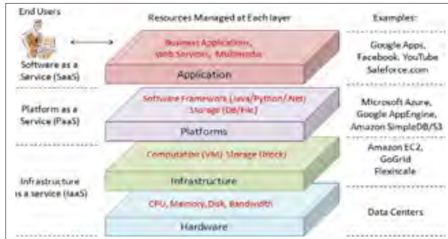
Figure 1.1 Cloud Computing Architecture Overview. (Zhang et al. , 2010)
