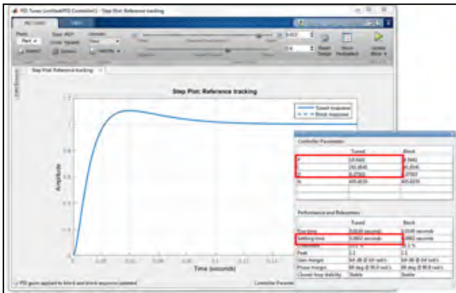
Figure 3.32 PID controller tuning using MATLAB/Simulink toolbox
