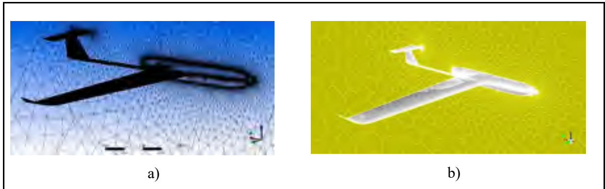
Figure 4.8 Tetrahedral mesh (a), Polyhedral mesh (b)
