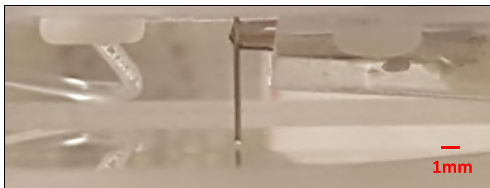
Figure 4.6 : Fluid preload, hemisphere droplet at end of dispensing needle
