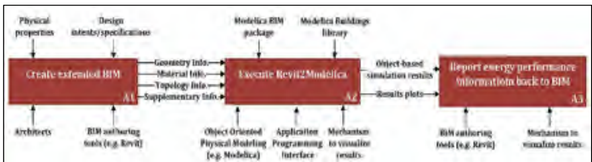
Figure-A I-2 Overall BIM to BEM process map for Revit to Modelica
