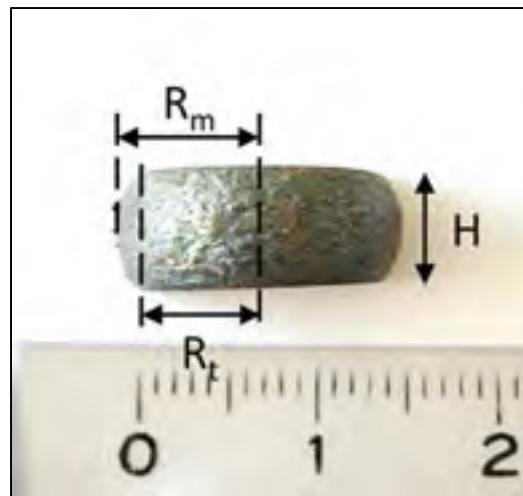
Fig. 4 Sample after hot compression test at 1223K and 0.01s^{-1}
