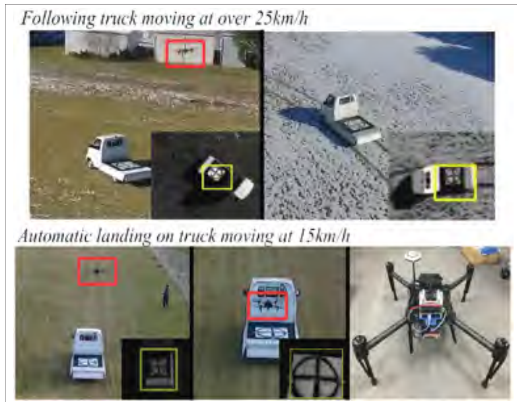
Figure 1.26 The yellow bounding box indicates the results of our tracking. Red box is the position of the flying uav. Reference: Chaudhary et al. (2017) page 1
