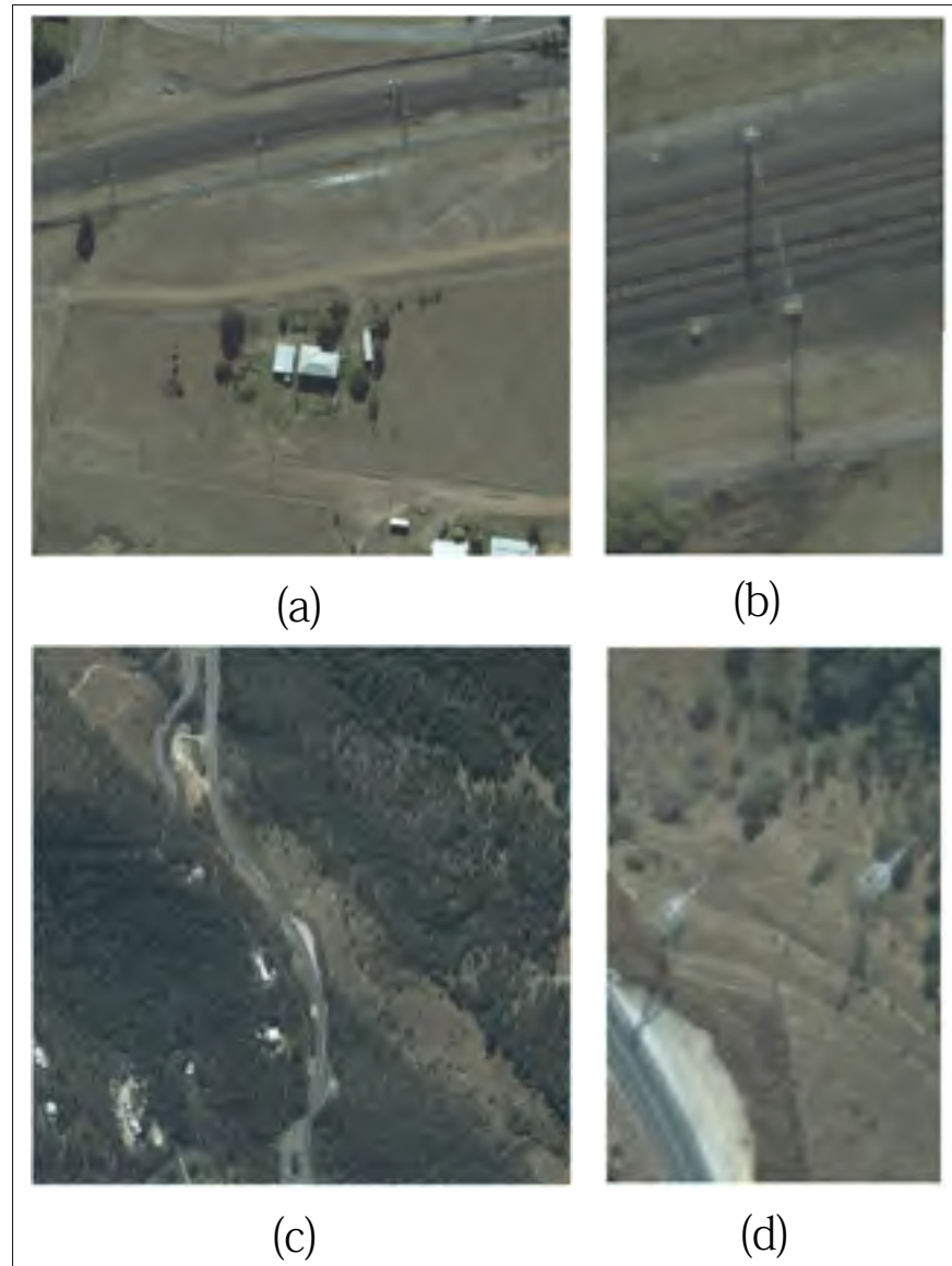
Figure 1.4 a) Rural area image with visible pole shadows around the dirt roads and rail tracks, b) Close up views of rail poles, c) Rural area image with electricity poles and pylons. d) Close up views of electricity poles or pylons. Reference: Pontecorvo & Redding (2017) page 5
