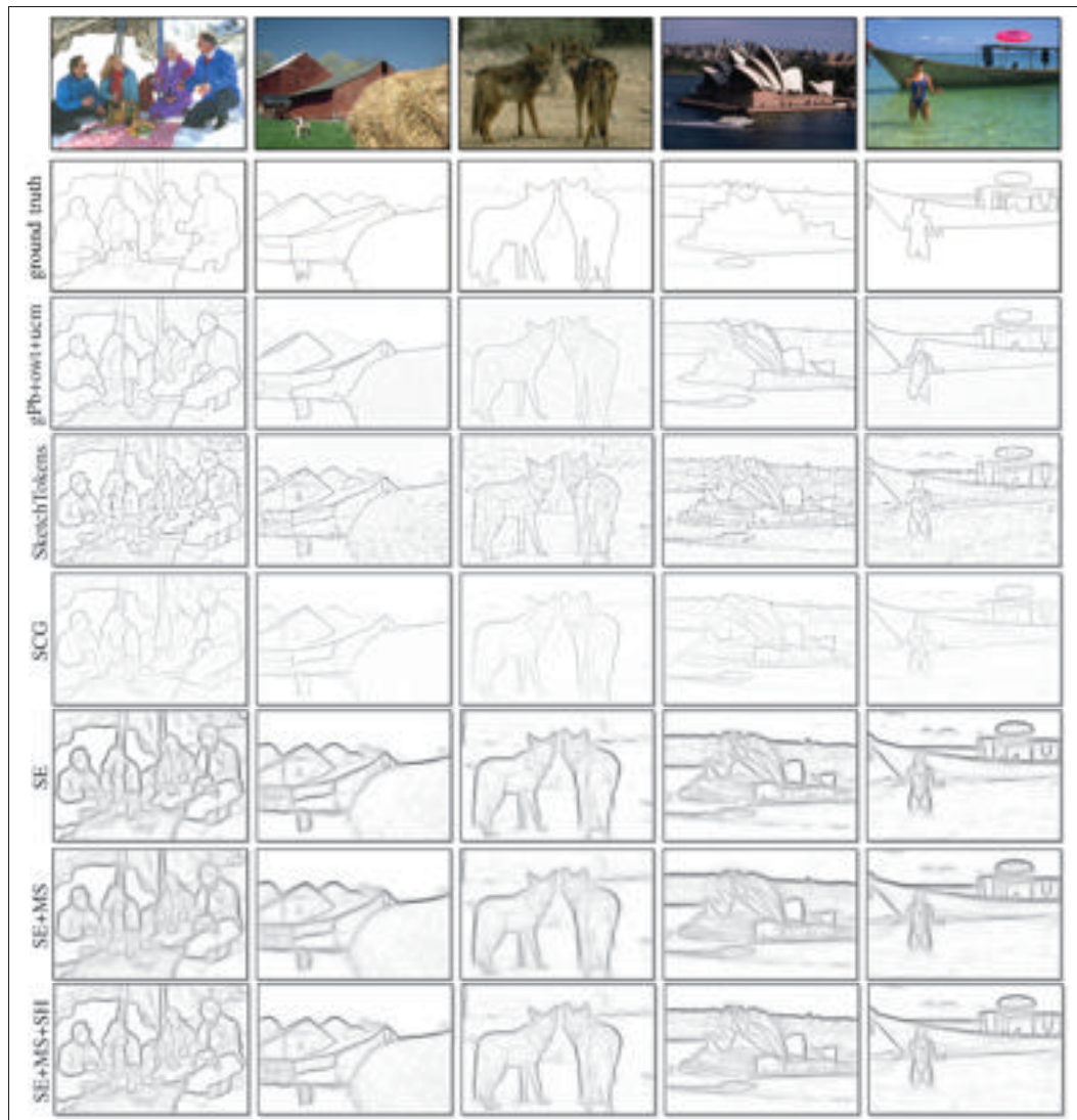
Figure 1.7 Results of edge detection on the BSDS500 dataset on five different sample pictures. The first row is the original image, the second row is ground truth. The third row show results for gPb-owt-ucm. The next two rows demonstrate results for Sketch Tokens, and SCG. The last four rows contain proposed results for variants of SE. Reference: Dollár & Zitnick (2015) page 6
