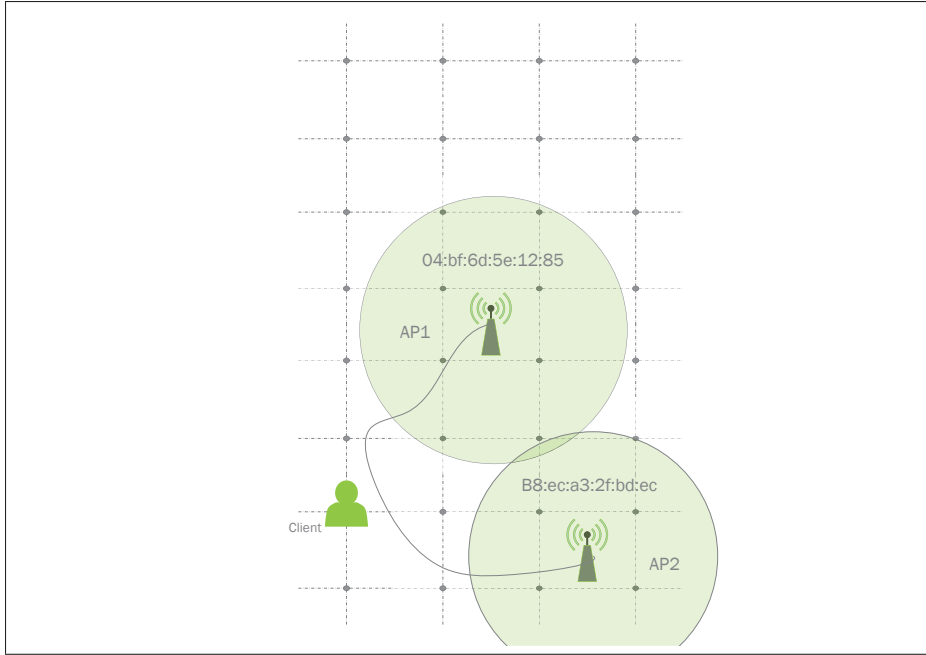
Figure 5.1 In access point to access point you can see different MAC address at two different APs.
