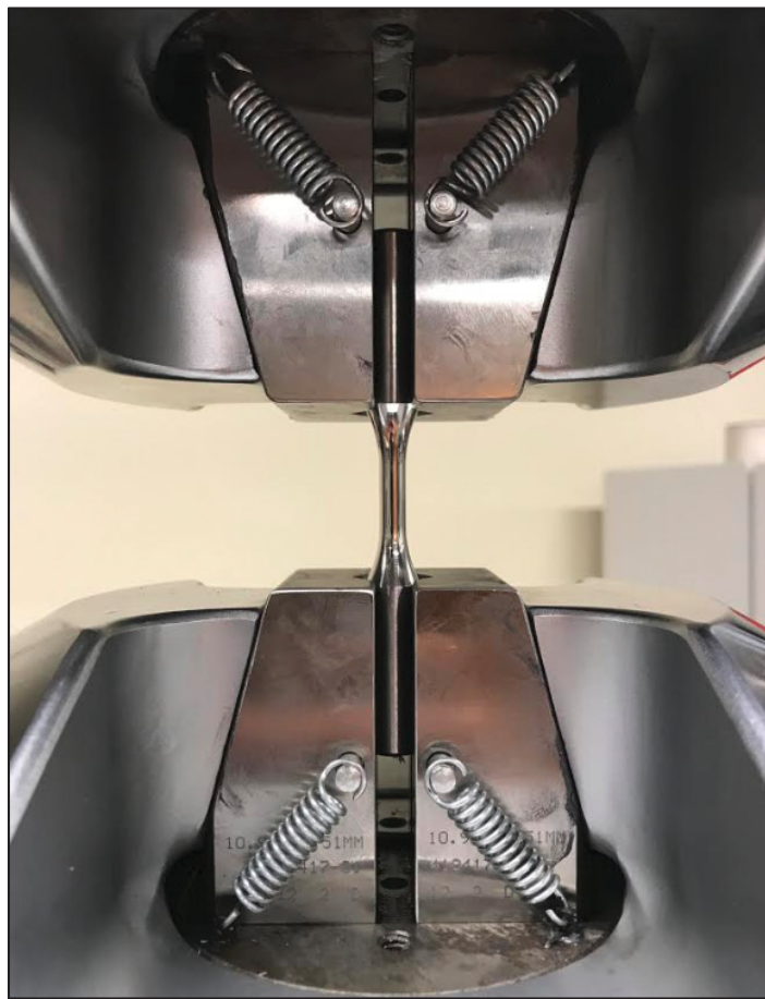
Figure 4.6 Fatigue specimen mounted for testing
