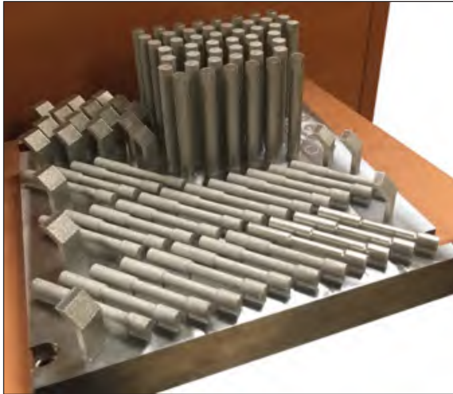
Figure A 2: Image of the build plate with 0° and 90°-oriented tensile blanks series
