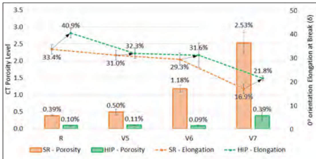
Figure A 11: Porosity (Archimedes') and elongation at break for R, V5, V6, and V7 specimens before and after HIP
