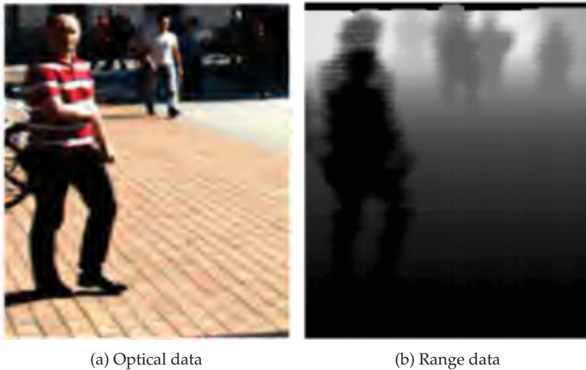
FIGURE 1.1: In the scenario of pedestrian detection, (a) optical data can provide useful RGB information while (b) range data can provide useful distance information. Data from different sensors can provide complementary information to improve the detection performance. This figure is extracted from [186].
