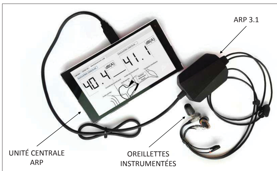
Figure 3.5 Configuration de base de la ARP 3.1, tirée de CRITIAS, NSERC-EERS Industrial Research Chair in In-Ear Technologies (CRITIAS)
