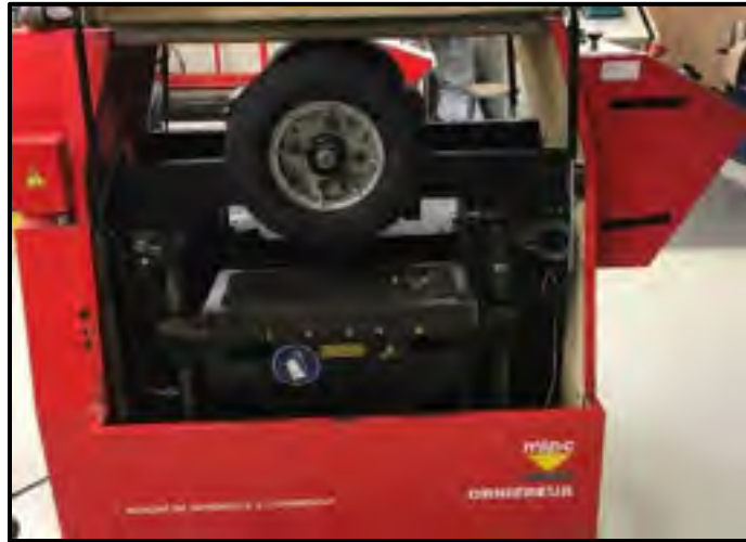
Figure 3. 3 Specimen preparation for the rutting tests
