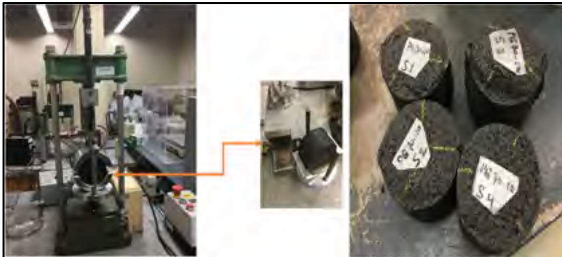
Figure 4. 2 Marshall testing machine and sample setup
