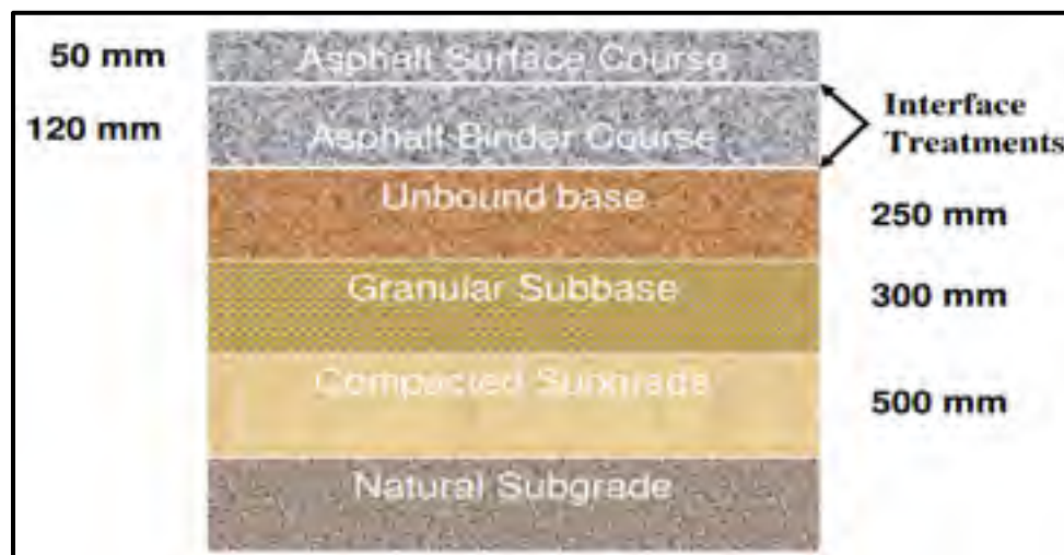
Figure 1. 4 Cross section of a typical ACP Taken from Jenks et al. (2011)
