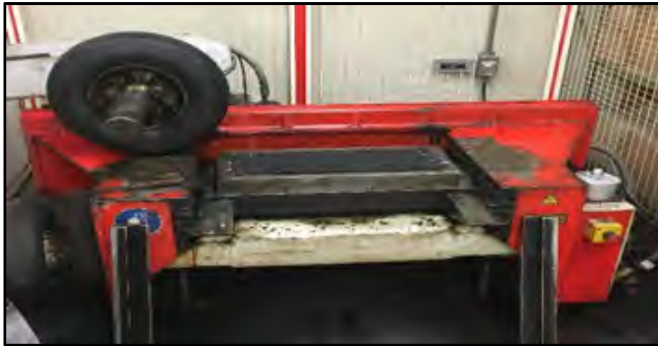
Figure 4. 3 French laboratory slab compactor LPC
