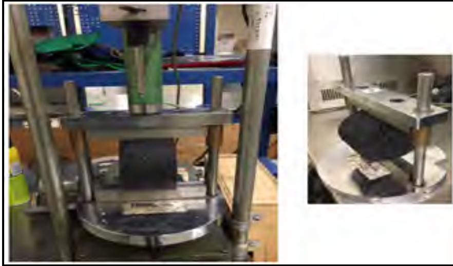
Figure 5. 7 ITS measurement system and sample setup
