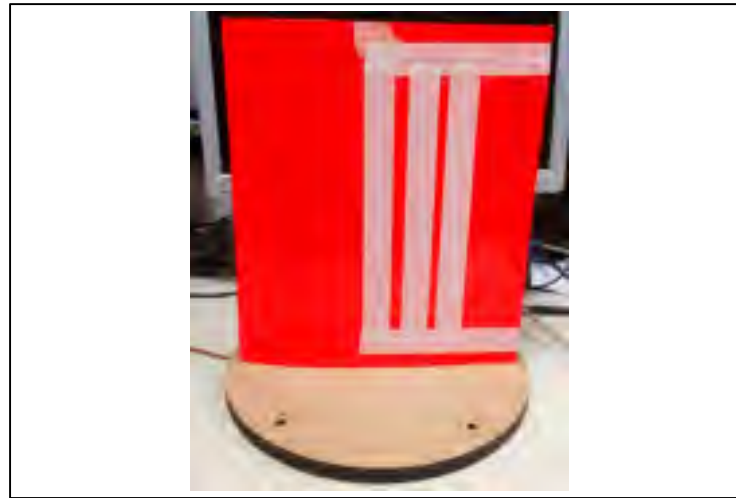
Figure 3.20 Experiment 1 with all slits covered by tapes (continuous surface)
