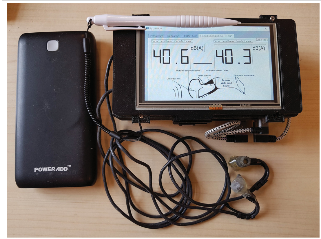
Figure 2.1 Picture of the developed system (ARP3DPOAE) with the additional external battery supply, touch screen stylus and earpieces showing measured OEM and IEM sound pressure levels. The external battery provided enough energy for 8 hours
