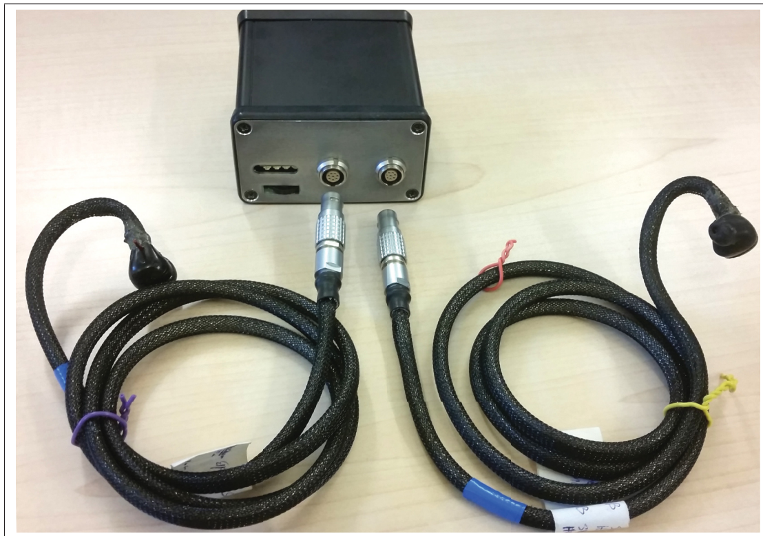
Figure 3.1 The distortion product otoacoustic emission measurement device designed in a laboratory with its electronic hardware box and its two measurement probes featuring custom-molded ear tips
