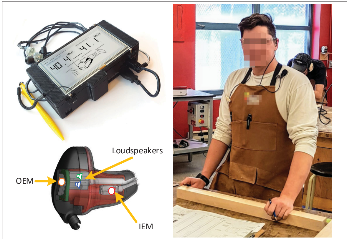
Figure 4.1 The Auditory Research Platform (ARP) with hearing protection earpieces including electronic components for outer-ear and in-ear noise dosimetry (left), and a worker wearing the ARP during in situ measurements (right)
