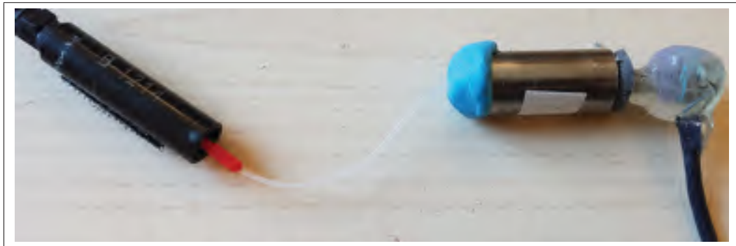
Figure 2.16 Setup used to compare the different sound pressure response measured in a test cavity simulating an earcanal with the DPOAE earpiece at the entrance and the probe microphone at the eardrum position
