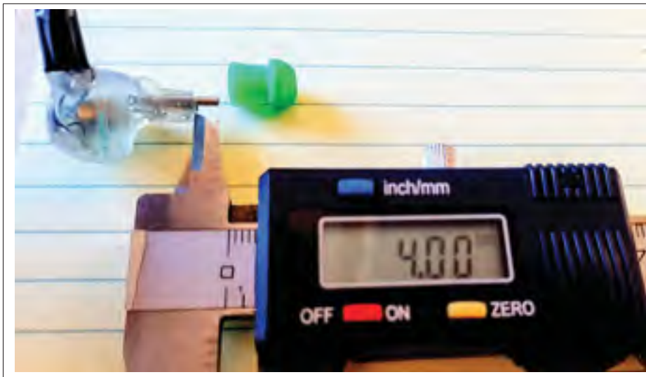
Figure 2.11 Earpiece for FPL calibration with loudspeakers' metal tubes cut flush with the plastic underbody shown with the green silicone eartip . The IEM metal tube protruding by 4 mm compared to the loudspeakers' tubes helps to minimize evanescent waves
