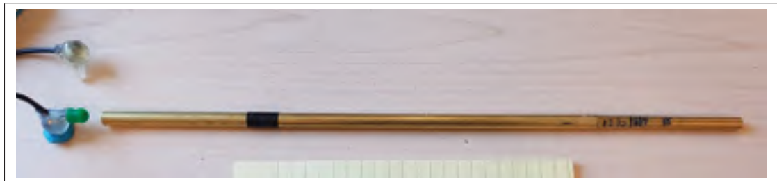
Figure 2.13 Picture of the cavity with variable lengths achieved with the sliding piston with a very precise outer diameter that fits snugly in the inner diameter of the brass tube. The piston needs to be at least approximately 10 cm in the tube to allow sufficient acoustical seal for FPL calibrations
