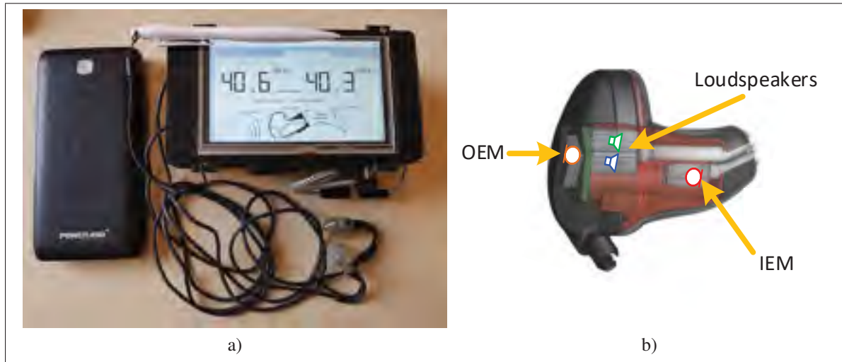
Figure 5.1 a) Designed system with DPOAE earpieces also used as hearing protection with foam eartips. b) Each earpiece includes in-ear/outer-ear microphones and two-miniature loudspeakers for DPOAE stimuli generation
