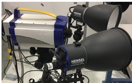
Figure 2-10 IRT reflection setup
