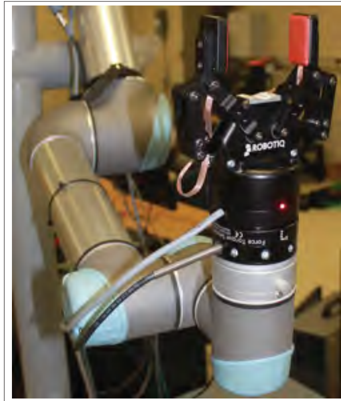
Figure 3.15 Close-up on the new setup used to study generalization: new tactile sensors (dynamic + accelerometer), gripper and UR5 robot
