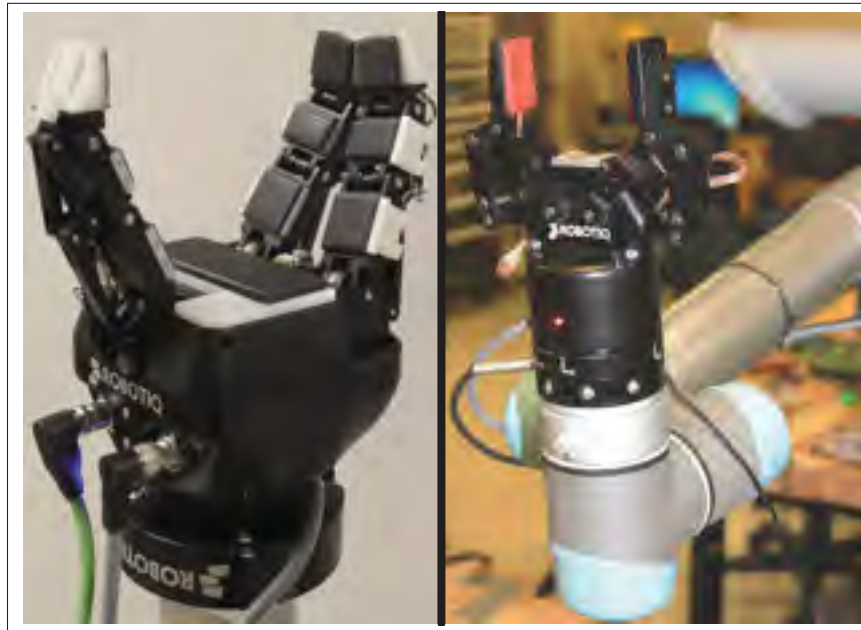
Figure 3.2 The two setups used during the experiments: a) on the left, a Robotiq 3-finger gripper equipped with our lab’s 1st-gen tactile sensors mounted on a UR5 robot and b) on the right, a Robotiq 2-finger gripper equipped with our 2nd-gen tactile sensors, mounted on a different UR5 robot
